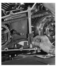
For proper spring tension, the distance between the guide plate and the bottom of the shoe should be 3/8".
