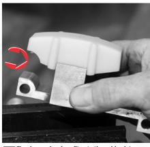
The shoe and springs fit onto the guide plate as shown, with the curved relief in the shoe (arrow) facing the front of the bike.
