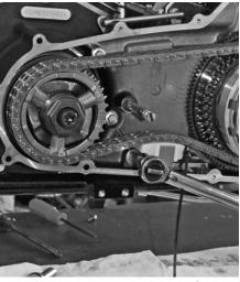
Tighten the Loctite-prepared stock 3/8" bolts to 21-24 ft-lbs.
