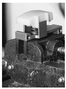
Here's the assembled M6 tensioner. If required, the supplied adjustment shims will be installed later.
