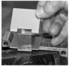
If needed, one or both of the supplied shims can be inserted under the shoe to correct the installed spring height. Try the thin one first.
