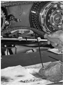
As directed in the H-D service manual, capture the original tensioner with a wire-tie to ease removal. Gently levering up the chain with a screwdriver will make inserting the wire-tie
