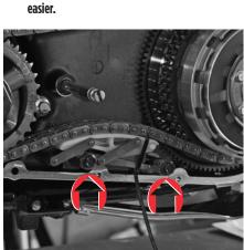
With the original tensioner captured, removing the two 3/8" bolts (arrows) that secure the tensioner to the inner primary cover and easing the tensioner out should be a breeze.
