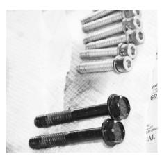
After a thorough cleaning and a drop of 242 Loctite, the original bolts will be used to install the new Hayden M6 tensioner.
