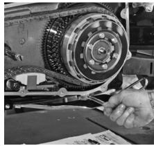
The drain plug was wrapped with Teflon tape at the factory. I followed suit after installing a new 0-ring. Tighten the plug to 14-21 ft-lbs.
