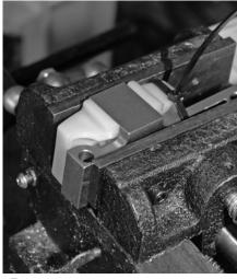
After putting the M6 tensioner sideways in the vise, carefully compress it and then capture it with a tie-wrap, which should insure a painless installation.
