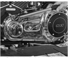
After insuring that the long and short screws go where they belong and have each gotten a drop of Loctite 242, tighten them to 12-13 ft-lbs.
