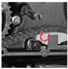
Yep, the curved relief in the bottom of the shoe (arrow) faces forward to clear the front mounting bolt.
