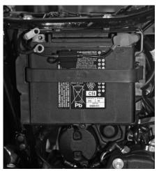
But before removing the primary cover, disconnect the cables from the negative (-) side of the battery. Use a #2 Phillips screwdriver to remove the battery cover and a #3 Phillips to disconnect the cable.
