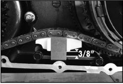
NOTE: The 3/8" is measured from the bottom of the shoe to the resting point of the springs on the guideplate, or shims (closest to the vertical bars).
