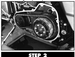
Remove the factory primary chain tensioner, along with any spacers that may be included on the back side. Keep the two stock bolts for the installation of the M6.
